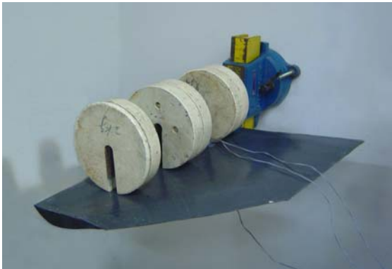
Fig. 13. Static structural test setup of the sub-scale wing loaded by the simulated aerodynamic load with three steel weights
