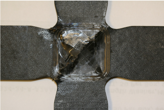
Fig. 3. Thickness-Tapered Cruciform Specimen Failure Surface when Subjected to -1/-1 Loading Conditions.
