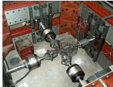
Fig. 1 Biaxial test bench developed at the VUB
