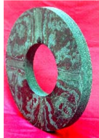
Fig. 5. C/C brake (diameter 40 cm) densified by Film Boiling process.
