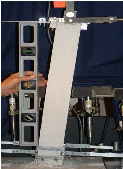
Fig. 3. Large inelastic deformations of bridge pier samples during testing
