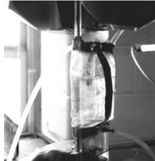
Fig. 3. Fluid cell used to insure continual saturation and temperature during fatigue testing
