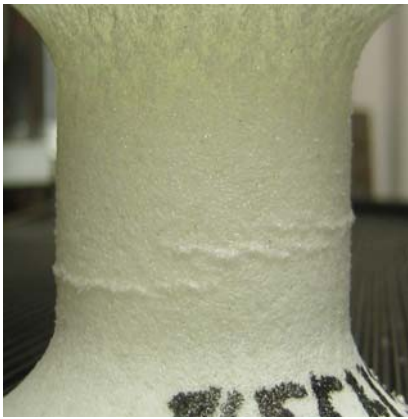
Fig. 7. Photograph of compression-compression fatigue test specimen showing typical crush band fracture in compression fatigue.
