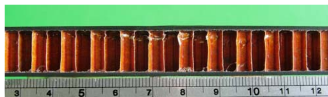
Fig. 4 A nomex sandwich panel impacted at 16 J
