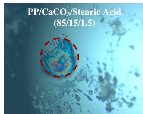
Fig. 1. Optical micrograph of the silicon nitride counterface after wear testing on polypropylene/calcium carbonate (85/15) nanocomposite having 1.5 phr stearic acid showing the presence of a thin, stable and uniform film.
