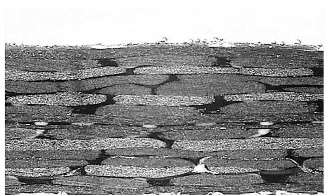
Fig. 1. Typical NCF composite microstructure,  $[0/90/45/-45]_{S_2}$ .
