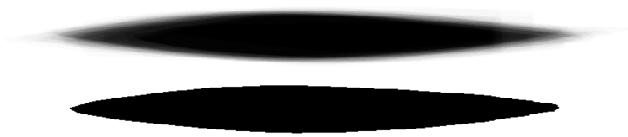
Fig 5. Sum of 80 outlined yarn cross sections for a 2 layer plaque made with Vetrotex RT600 in grayscale and binary.
