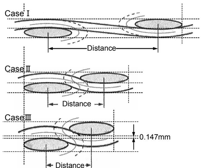
Fig.9 Schematic drawing of braiding structure.
