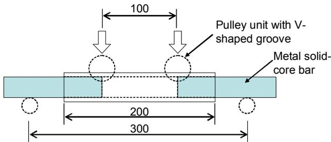
Fig 4. Schematic drawing of 4-point bending test.
