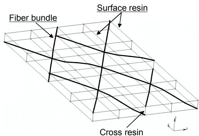
Fig.6 Weaving structural model
