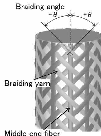
Fig.1. Schematic drawing of braided fabric.
