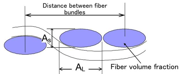
Fig 3. Schematic drawing of the cross-section along the braiding yarn.
