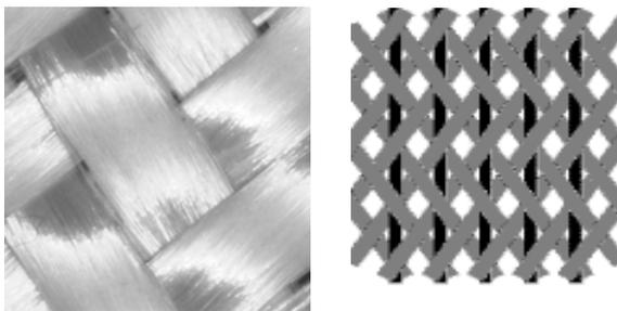
**Figure 1 Biaxial and Triaxial Braid Patterns**
