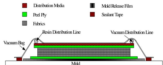
**Figure 2. Schematic Drawing of VARTM[1]**
