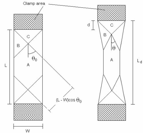
Fig. 1. Bias extension test with idealised shear zones (PJN assumption) for  $[\pm 45]$ ; undeformed and deformed specimen (illustration inspired by [2, 7])
