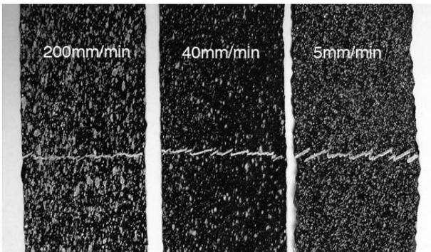
Fig. 6. Different cross-head rates tested at 70°C; the initially straight lines show the difference in slip
