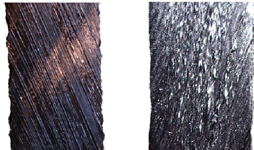
Fig. 8. Comparison of the wrinkling mode at 70°C (to the left) and at RT
