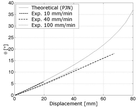
Fig. 7. Theoretical fibre rotation compared with experimental results for  $[\pm 45]_s$ ; at 70°C with different cross-head rates
