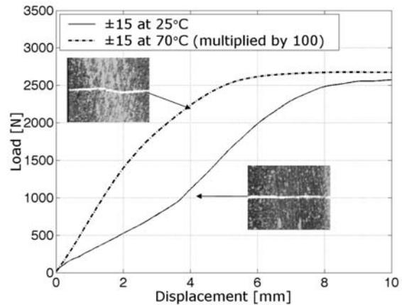
Fig. 10. Typical curves for  $[\pm 15]_s$  with a cross-head speed of 13 mm/min, tested at 25 and 70°C (note that load is multiplied by 100 at the elevated temperature)
