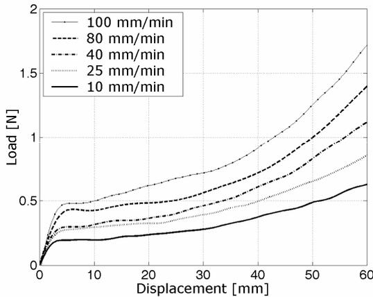
Fig. 5. Different cross-head rates tested at 70°C
