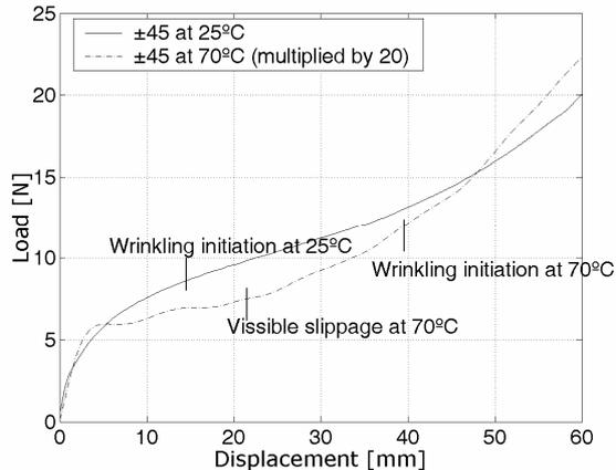
Fig. 9. Typical curves for  $[\pm 45]_s$  with a cross-head speed of 40 mm/min, tested at 25 and 70°C (note that load is multiplied by 20 at the elevated temperature)
