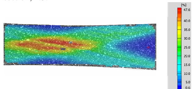
Fig. 4. Strain fields after a deformation of 2.5 mm for an initial cross-ply angle of 15
