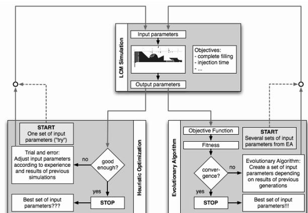
Fig. 1. Comparison of process optimization using an heuristic approach or evolutionary algorithms
