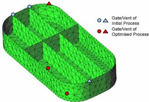
Fig. 6. Initial and optimized locations of gates and vents
