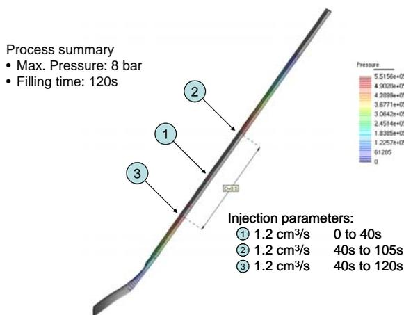
Fig. 3. Optimised impregnation process
