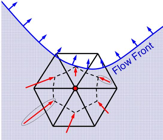
Fig. 4. flow velocities in elements connected to completely filled flow front node
