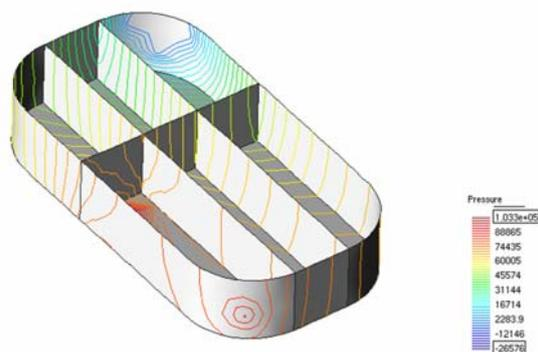
Fig. 7. Final pressure distribution of optimized process
