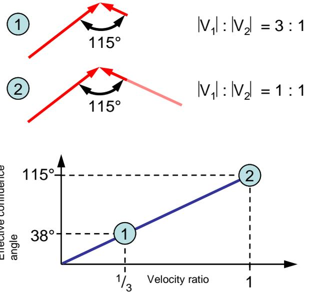
Fig. 5 effective confluence angle by linear scaling depending on the flow velocity ratio
