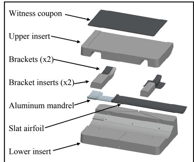
Fig. 11. Mould inserts for prototype slat
