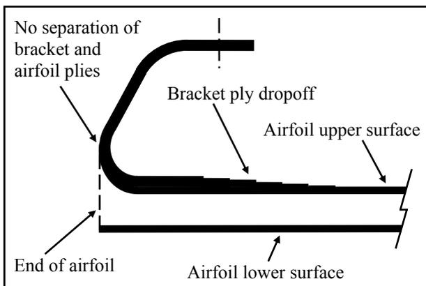
Fig. 4. Blended half bracket cross-section
