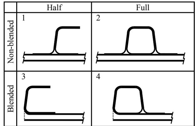
Fig. 5. Four possible bracket types
