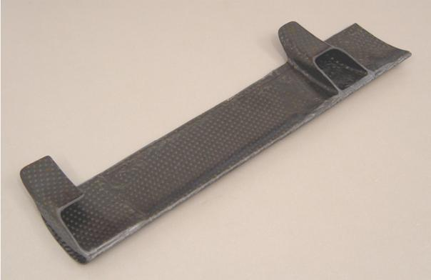
Fig. 15. Trimmed prototype slat
