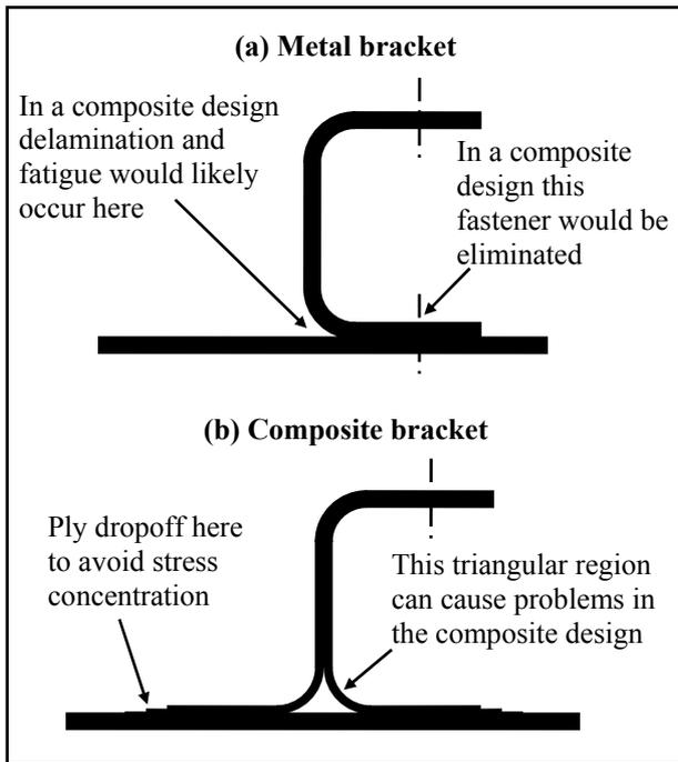
Fig. 3. Composite versus metal bracket design
