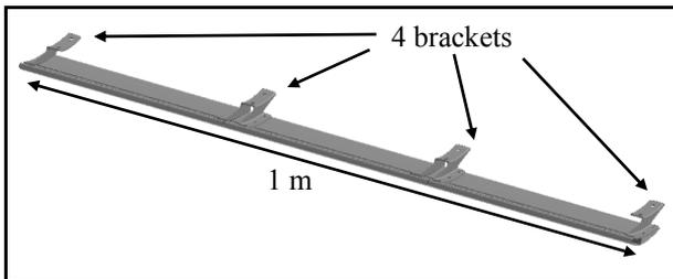
Fig. 1. Leading edge slat with attachment brackets
