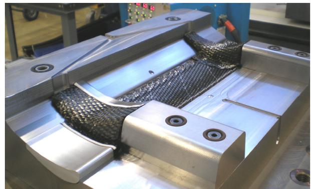
Fig. 13. Preform in the mould
