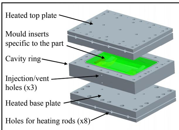
Fig. 10. Modular mould
