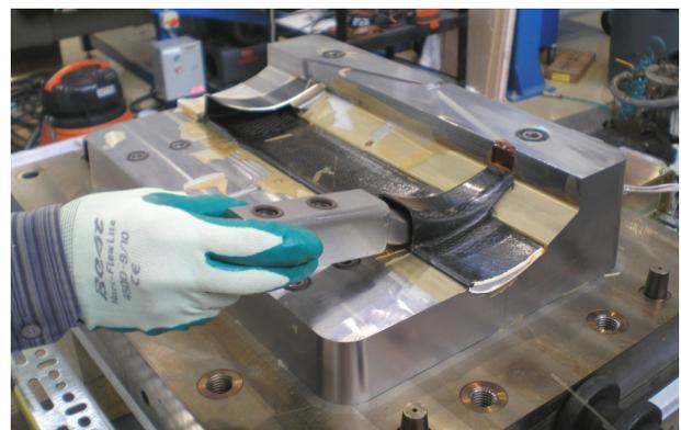
Fig. 14. Removing the full bracket insert after cure
