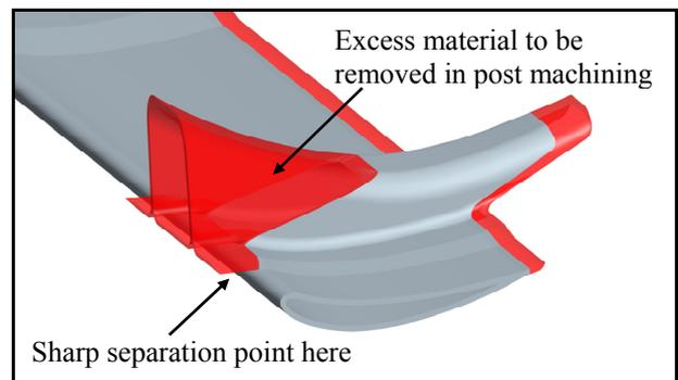
Fig. 6. Excess material along all part edges
