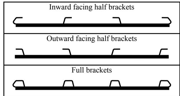
Fig. 2. Examples of possible bracket configurations
