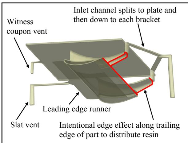
Fig. 12. Mould cavity to be filled
