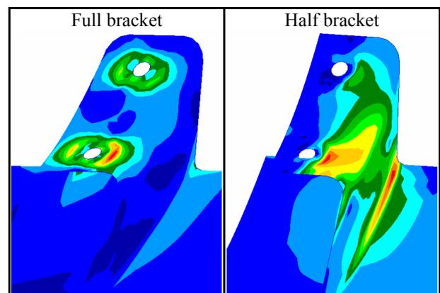
Fig. 8. Sample FEA results showing stress concentrations at bracket holes and radii
