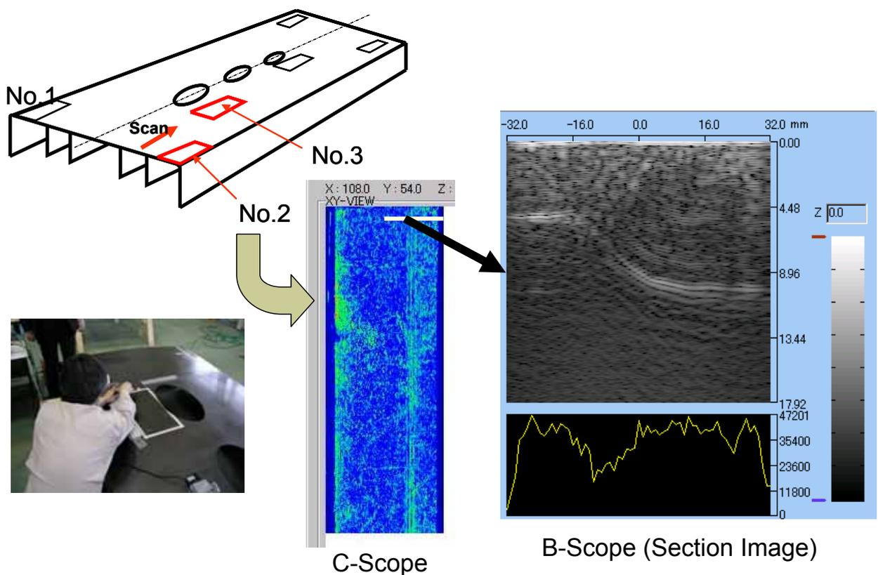
Fig. 8. Results of 3-D Ultrasonic Scan of part No. 2.
