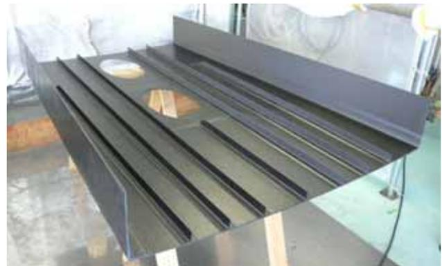
Fig. 2. Picture of an experimental production of lower wing panel integrated with spars and stringers by VaRTM process. (2.1 m X 1.4 m)
