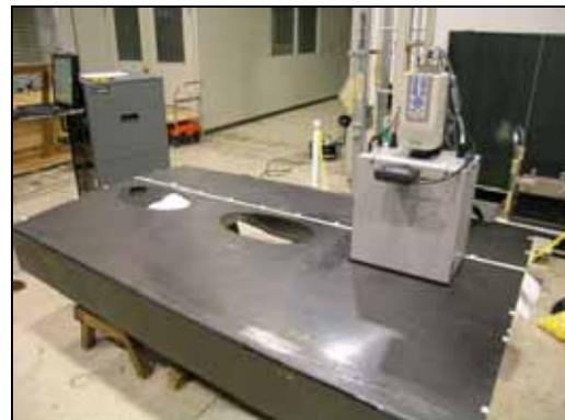
Fig. 3. Picture of inspection of 2 m VaRTM specimen by pulsed thermography.
