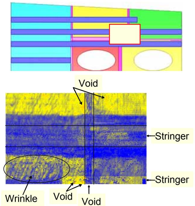
Fig. 7 Result of Ultrasonic C-Scan of thick part.
