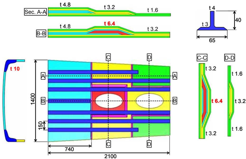
Fig. 1. Schematic illustration of thickness distribution in 2.1 m-span lower wing panel with stringers and maintenance holes.
