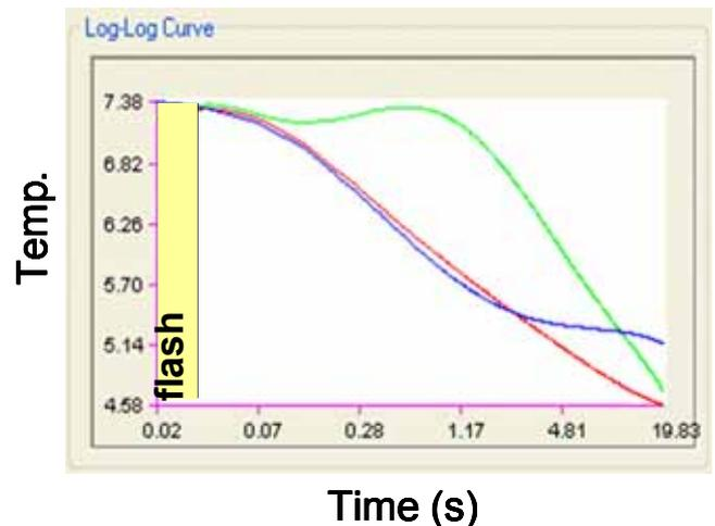
Fig. 6 Log-Log plot of surface temperature time history on the specimen at the marked points in Fig. 5.
