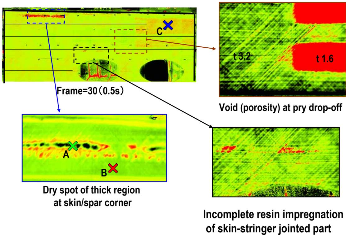
Fig. 5. NDI result of pulsed thermography.
