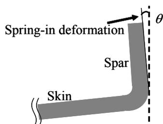
Fig. 6. Definition of spring-in deformation
