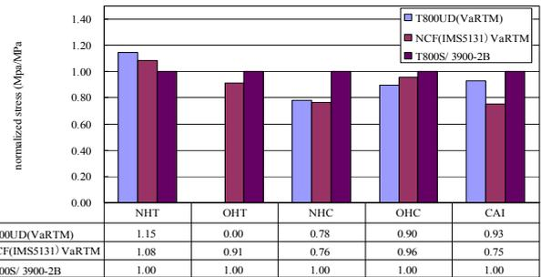
Fig. 2 Mechanical properties of Va-RTM composite (normalized by conventional prepreg composite properties)
