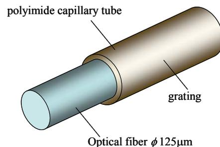
Fig. 10 Encapsulated FBG sensor
