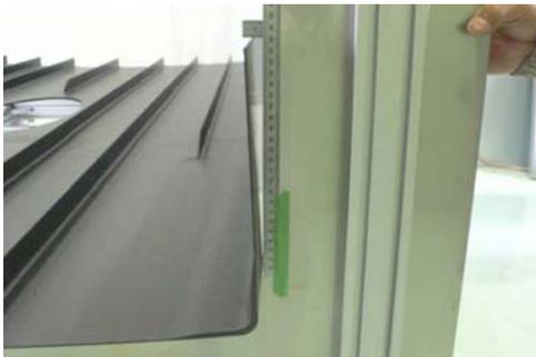
Fig. 5. Spring-in deformation of 2.1m long demonstrator
