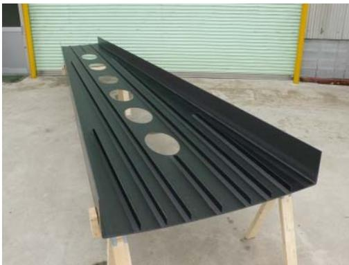
Fig. 4. 6.0m long wing-box demonstrators
