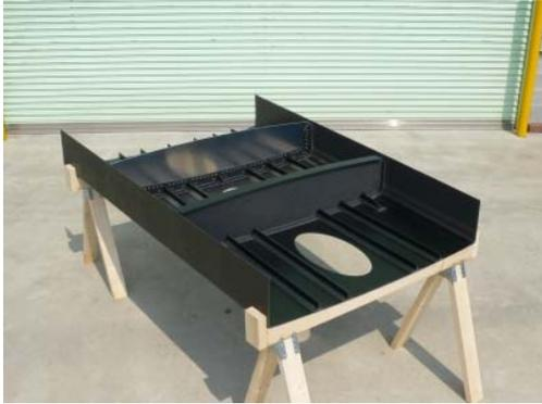
Fig. 3. 2.1m long wing-Box demonstrators
