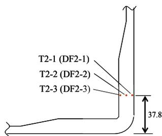
Fig. 9 Thickness location of the embedded sensors
