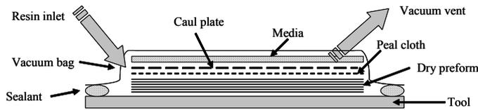
Fig. 1 Schematics of Va-RTM process
