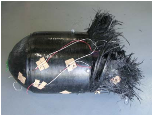
Fig.14 Busted condition of filament winding vessels
