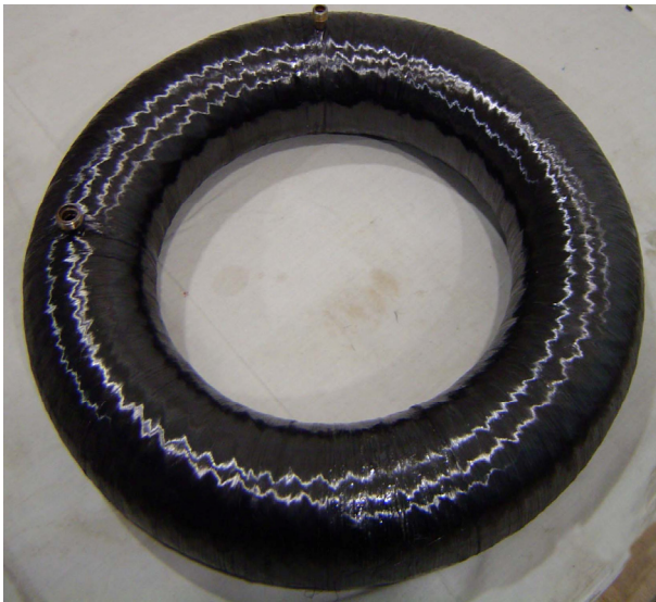
Fig. 11. A finished toroidal pressure vessel wound by non-geodesic pattern
