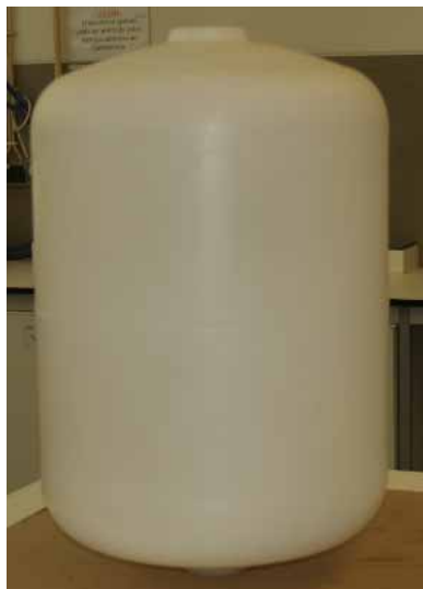
Fig. 2. Rotational moulding HDPE liner
