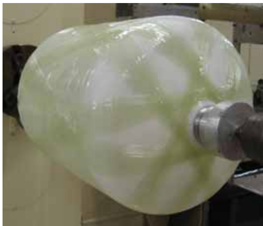
Figure 13 On-going prototype filament winding
