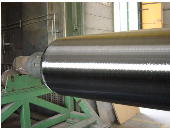
Fig.4. Mandrel wound without hardener enters the oven
