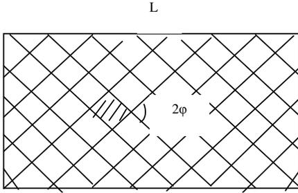
Fig. 7 The non-deformed structure of fibers on the cylinder
