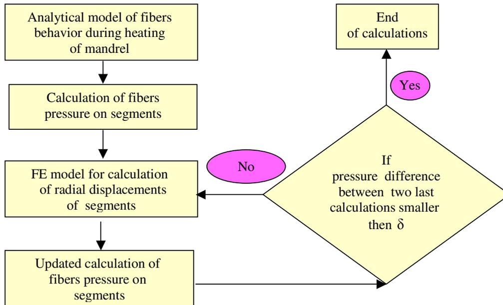
Fig.12 An iteration process of calculations
