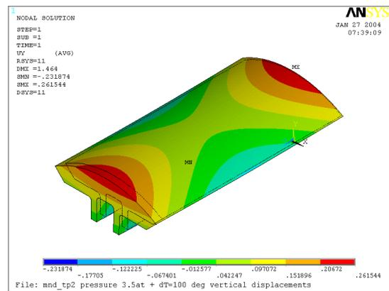
Fig.13 Vertical displacements of the segments of improved mandrel under external pressure and high temperature
