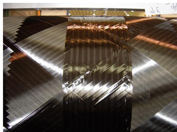
Fig.6. Wrinkles on the external hoop wound surface of the heated case in the heating test 2
