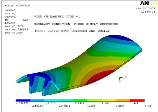
Fig.11 Vertical displacements of the segments of mandrel under external pressure and high temperature
