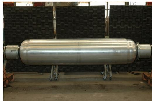
Fig. 2. Assembly of segmented mandrel
