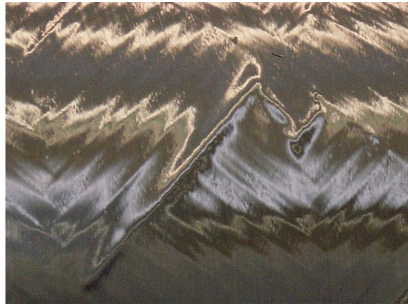
Fig.5. Wrinkles on the external surface of the heated case. Heating test 1
