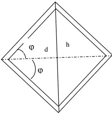
Fig. 9 Elementary rhombus of helically wound fibers before heating
