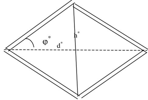
Fig. 10 Elementary rhombus of helically wound fibers after heating
