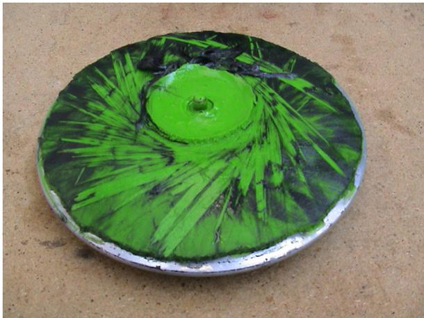
Fig. 12. Insert blown out of the pressure vessel
