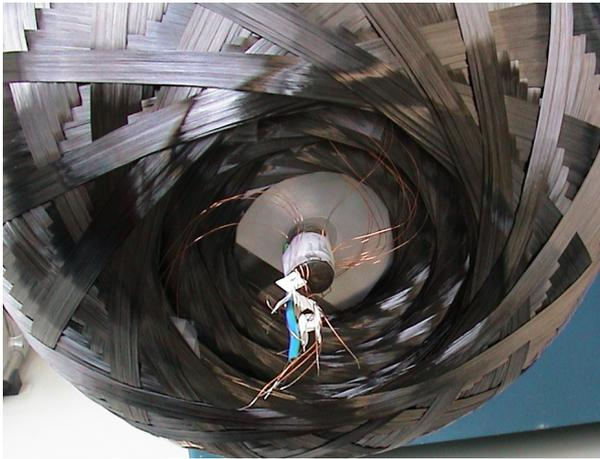
Fig. 8. Fiber stacking at the pole of a pressure vessel.
