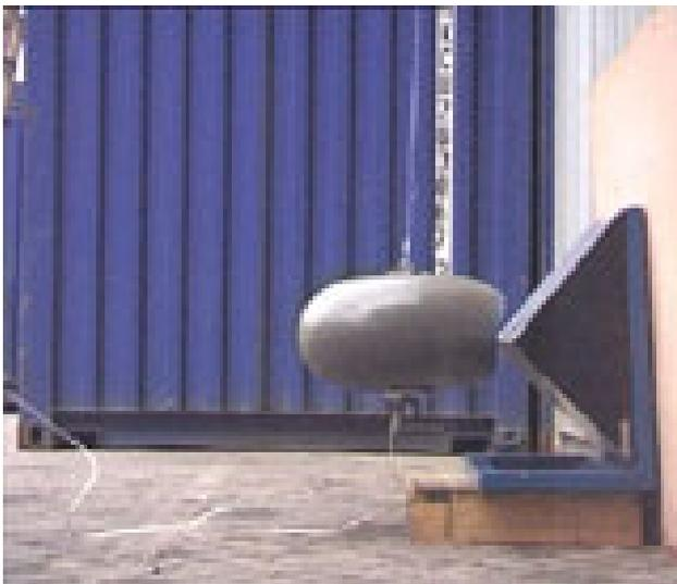
Fig. 2. Impact test on a LPG pressure vessel.
