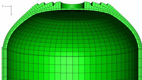
Fig. 9. FE element model for the layers (half of the model) shown at the poles.
