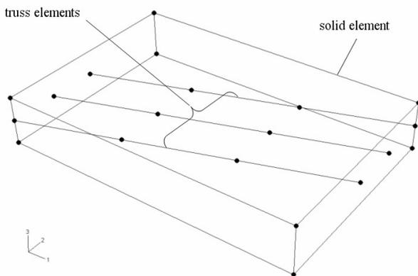
Fig. 6. Truss elements embedded in a solid element. The principle is used for modeling of dry wound fibers.
