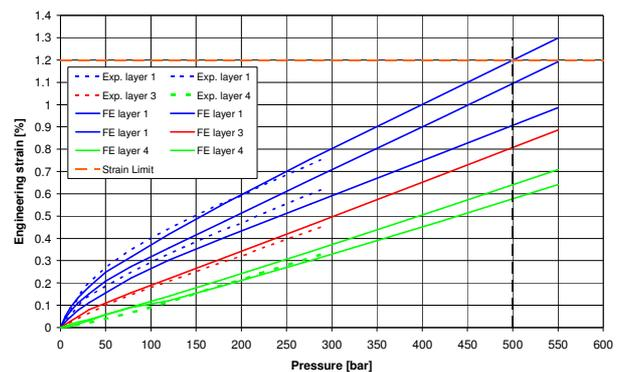
Fig. 14. Engineering strains as a function of the pressure for helix layer 1, 2 and 4 in experiment and for all helix layers in FE. The strain limit for Carbon Fiber Toray T700 24K is provided as well.
