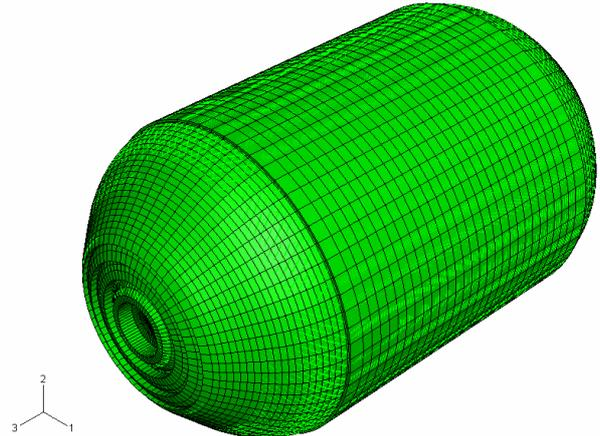
Fig. 5. FE model of a vessel with 4 helix layers and a hoop layer.
