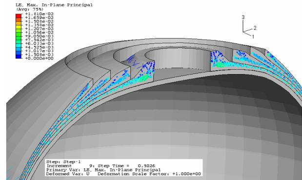
Fig. 13. Strain in the truss elements for a pressure of 276 bar.
