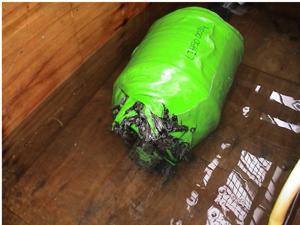
Fig. 11. Dry filament wound pressure vessel after burst test. Failure occurred at 495.3 bar.
