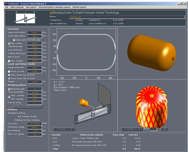
Fig. 3. Screen capture of the Graphical User Interface (GUI) of PresVes.
