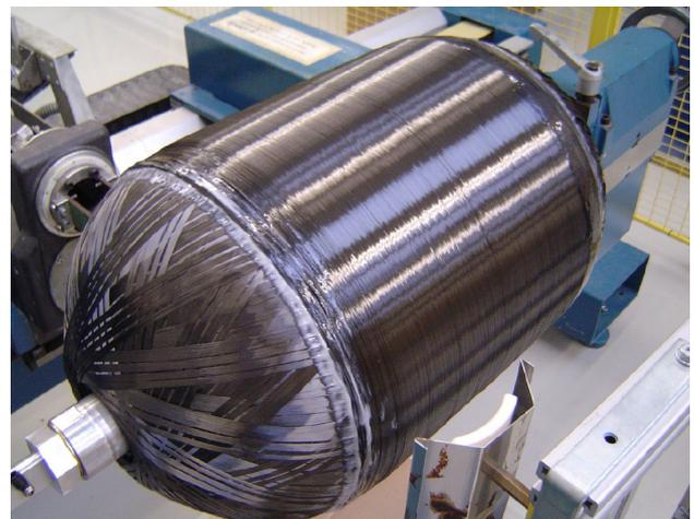
Fig. 1. Dry filament wound thick walled pressure vessel.
