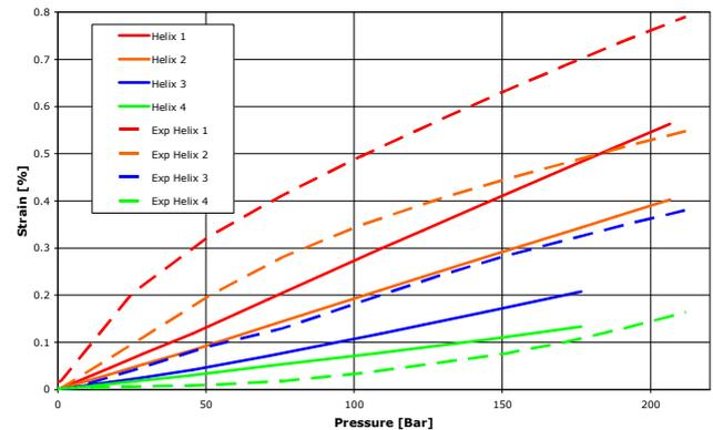
Fig. 7. Pressure-strain relations for a thick walled pressure vessel with 4 helix layers and a hoop layer.
