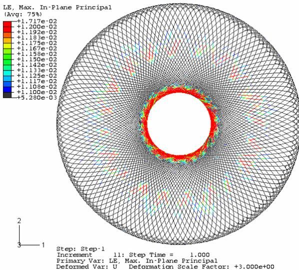
Fig. 15. Strain in the first helix layer at a pressure of 550 bar.
