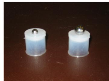
Fig. 3. Plastic sabots with steel ball impactors
