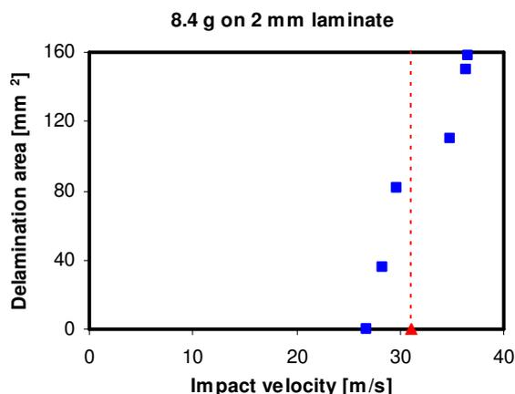
Fig. 6. Delamination size vs velocity for 8.4 g impactor on 2 mm laminate
