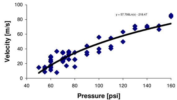
Fig. 9. Velocity scatter versus pressure for 8.2 g ball
