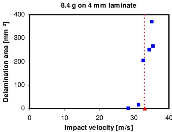
Fig. 8. Delamination size vs velocity for 8.4 g impactor on 4 mm laminate
