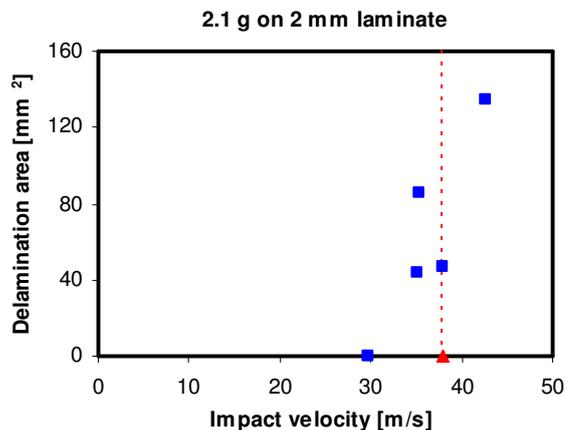
Fig. 5. Delamination size vs velocity for 2.1 g impactor on 2 mm laminate
