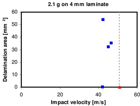
Fig. 7. Delamination size vs velocity for 2.1 g impactor on 4 mm laminate
