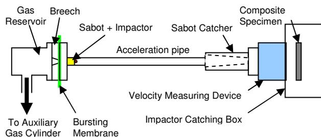
Fig. 4. Schematic drawing of gas gun
