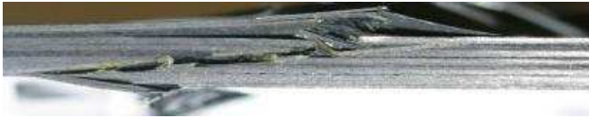
Figure 16 Failure location of the scarf joint with doubler specimen
