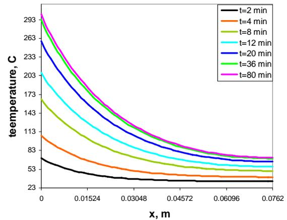
Fig. 9. Temperature variation in the direction of the current's flow in the middle plane of the cross-ply composite plate carrying a 50 A DC current
