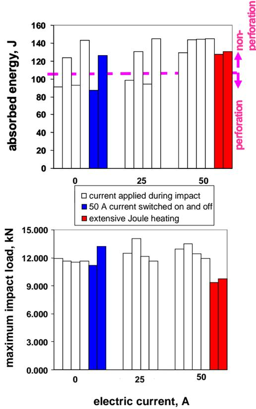
Fig. 7. Energy absorption and maximum impact loads as function of the electric current magnitude in low velocity impact tests on cross-ply composite plates
