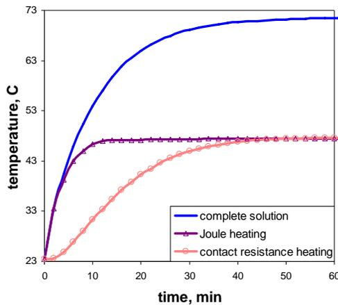
Fig. 10. Variation of temperature with time at the plate surface in the middle for the cross-ply composite plate carrying a 50 A DC current: effect of Joule heat and contact resistance heat
