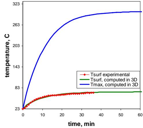
Fig. 8. Variation of temperature with time in the cross-ply composite plate carrying a 50 A DC current
