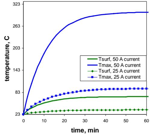
Fig. 11. Variation of temperature with time in the electrified cross-ply composite plate: the effect of the current's magnitude
