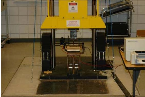
Fig. 1. GRC 8120 Drop weight impact test machine
