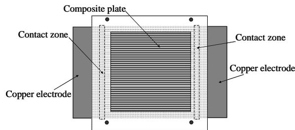
Fig. 2. Clamping fixture
