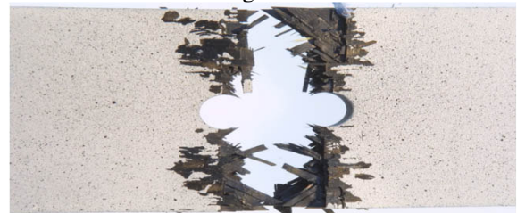
Fig. 3. Failure of a quasi-isotropic OHT specimen.
