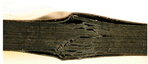
Fig. 7 Cross section view around the fracture (2Ti-32C-P).
