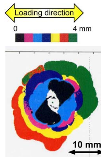
Fig. 14. C-scan image of the impacted side for the AS4/PEEK specimen at N=500, the impact-induced delaminations of which were shown in Fig. 4
