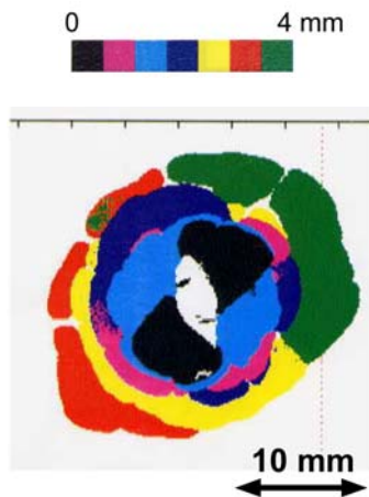
Fig. 4. C-scan image of the impacted side for an AS4/PEEK specimen subjected to 1.03 J/mm impact
