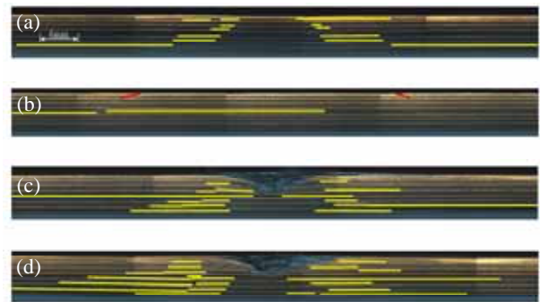
Fig. 8 Cross sectional observation for the impacted specimen by (a) hemispherical, (b) flat, (c) conical, (d) pyramid impactors
