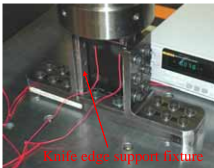
Fig. 4 Test apparatus for compression test after impact
