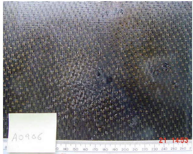
Fig. 5. 11% SMA laminate post Zone 1A lightning strike testing
