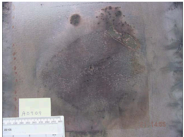
Fig. 6. Baseline laminate with Astrostrike surface layer protection post Zone 1A lightning strike testing
