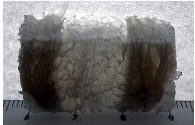
Fig. 6. Composite with a gradient of porosity and fibre fraction.
