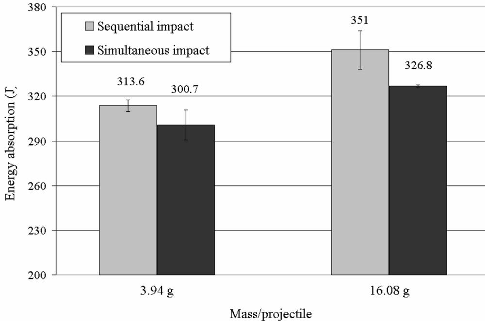
Figure 4. Impact energy absorption for thin S-2 glass laminates subjected to near-simultaneous and sequential impact by three Al<sub>2</sub>O<sub>3</sub> and tungsten carbide, .50 caliber (12.7 mm) diameter spherical projectiles
