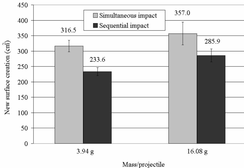
Figure 5. New surface creation (delamination) for thin S-2 glass laminates subjected to three projectile near-simultaneous and sequential impact by 3.94 g (Alumina/Al<sub>2</sub>O<sub>3</sub>) and 16.08 g (WC) .50 caliber (12.7 mm) diameter spherical projectiles.
