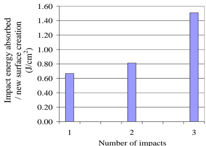
Figure 2. Impact energy absorbed/new surface creation (J cm<sup>-2</sup>) vs. number of sequential impacts showing an increase in damage area while the energy absorbed remained relatively constant.
