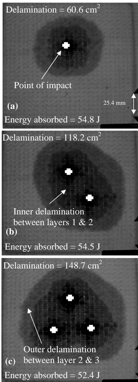
Figure 3. Sequential impact series with delamination damaged measured between impacts, (a) first impact, (b) second impact, (c) third impact.
