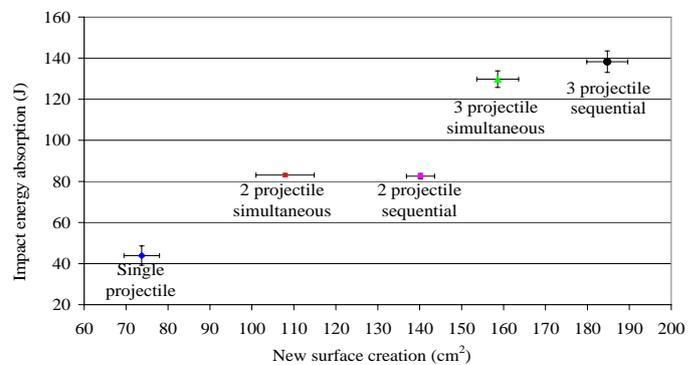
Figure 1. Impact energy absorption (J) vs. new surface creation (cm<sup>2</sup>) for single projectile, two projectile and three projectile impact series showing an increase in new surface creation for the sequential impact event.
