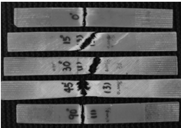
Fig 3. Failure modes of specimen of different orientations to the principal fiber.
