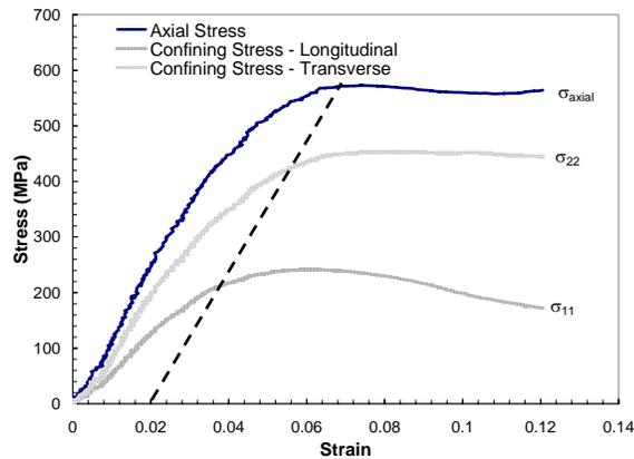
Fig. 2. A typical stress-strain curve for uni-directional fiber reinforced S-glass/epoxy composite under multi-axial loading.
