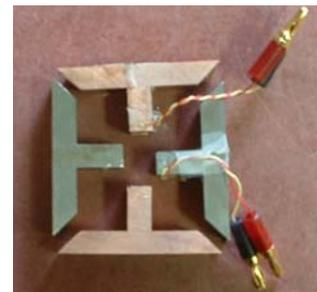
Fig. 1. Photograph of the instrumented biaxial confinement fixture for dynamic characterization of fiber reinforced composites.
