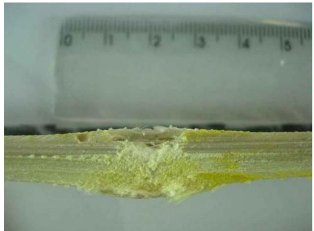
Fig.9 9 mm FMJ impact in a P2 nanocomposite
