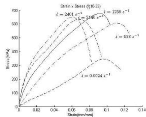
Fig. 3 Stress-strain curve for different strain rates – 10% nanoclay content
