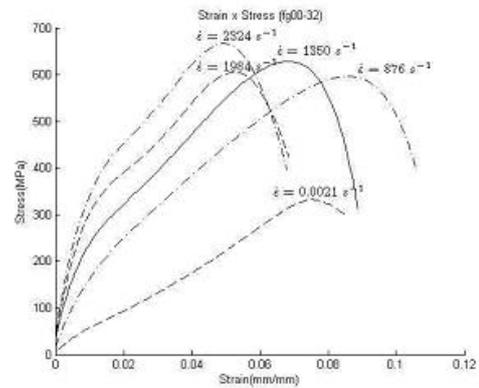
Fig. 1 Stress-strain curve for different strain rates – 0% nanoclay content
