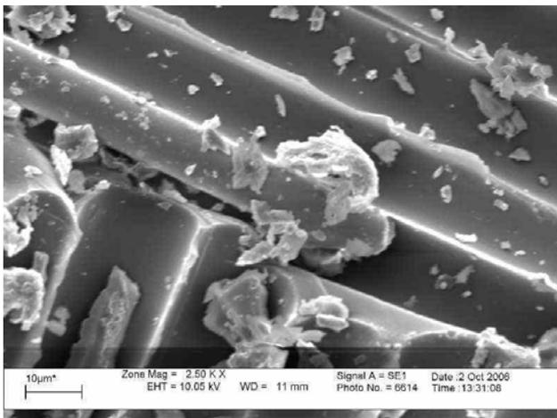
Fig. 4 SEM micrograph showing the nanocluster precipitation
