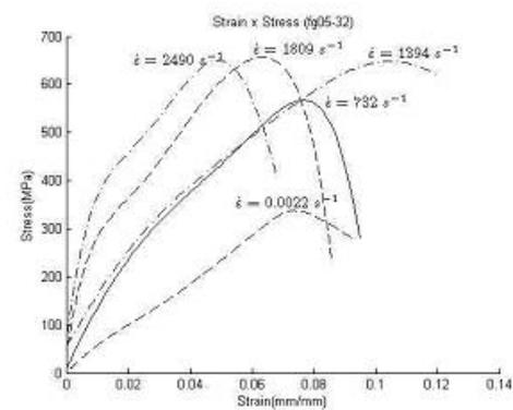
Fig. 2 Stress-strain curve for different strain rates – 5% nanoclay content
