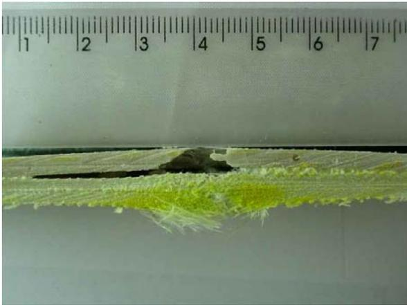
Fig. 7. 38 caliber impact in a P4 nanocomposite
