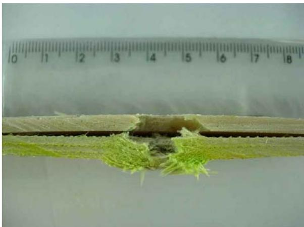
Fig. 8. 38 caliber impact in a P3 nanocomposite
