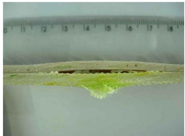
Fig.10 9 mm FMJ impact in a P4 nanocomposite
