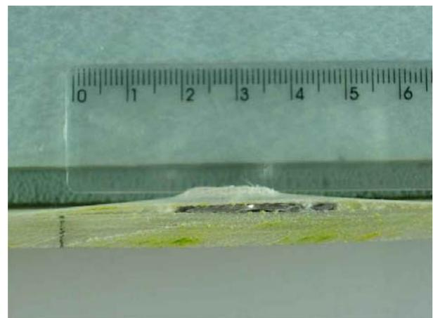
Fig 6. 38 caliber impact in a fiber glass/epoxy
