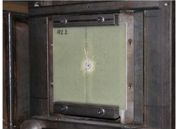
Fig 4. Impacted laminated panel in test rig
