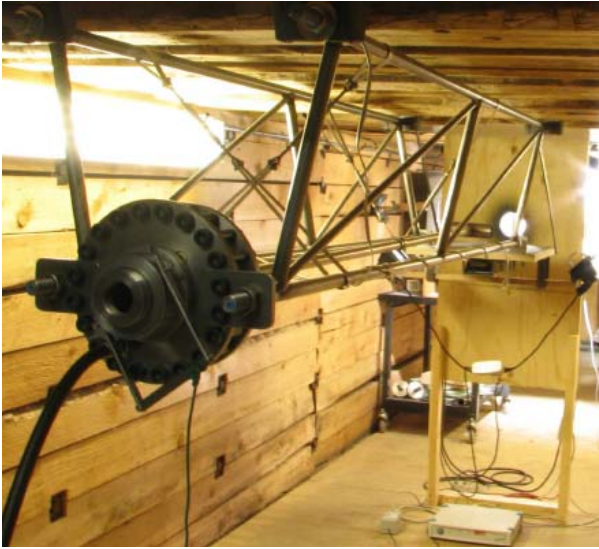
Fig. 2. The compressed air gun in the test chamber
