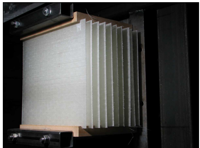
Figure 3: Test set up of 10 plates of 1 layer laminates
