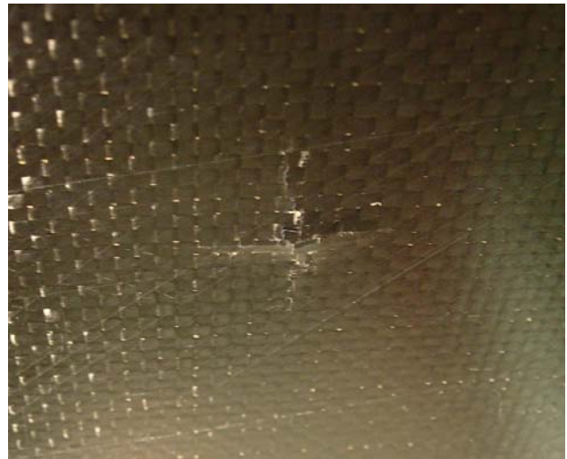
Fig. 7. Backside fiber failure for 25.4 mm cotton-filled ice at 71.6 m/s
