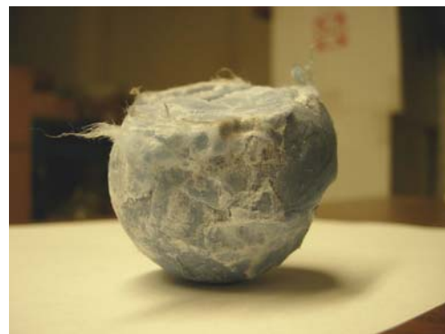
Fig. 8. Cotton-filled ice recovered after impact test showing formation of flattened spot
