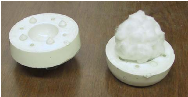
Fig. 3. Dry cotton fill (8 g) in 50.8 mm ice mold
