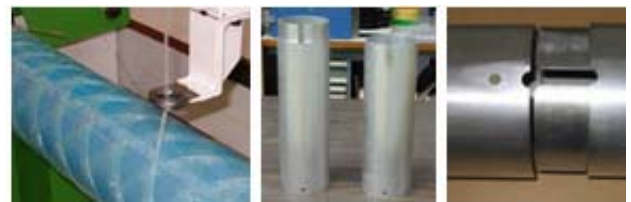
Fig. 11. Filament winding (left), split mandrel (center), and cable passage (right)
