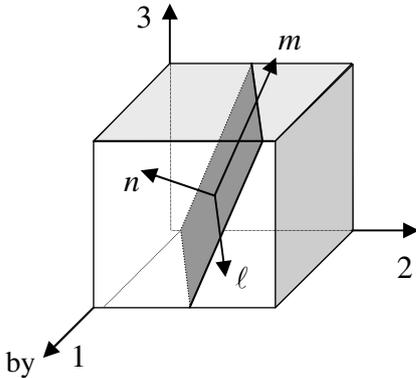
Fig. 2: Local coordinate system aligned with the crack
