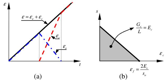
Fig. 3: (a) Elastic and crack components of the strain; (b) cohesive law and fracture toughness
