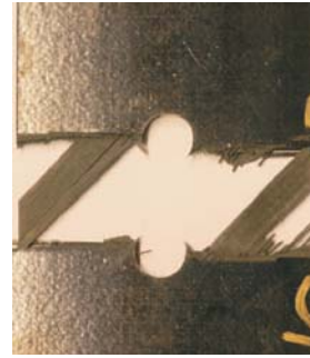
Fig. 2. Net-section tension failure mode.
