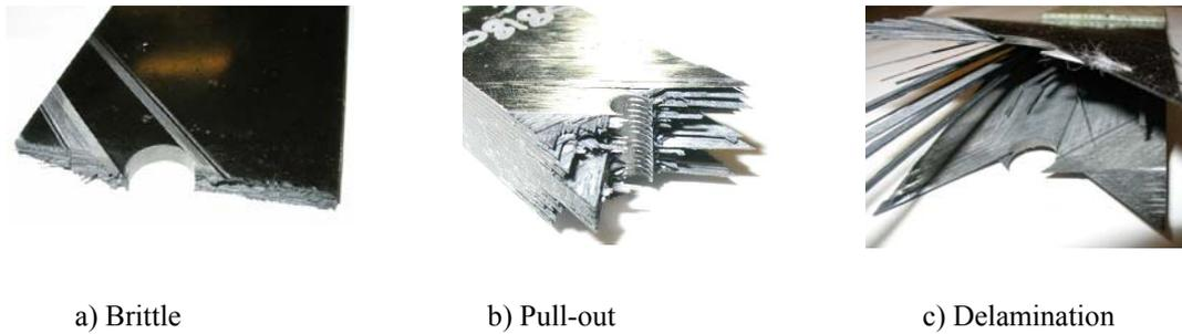
Fig. 3. Failure mechanisms
