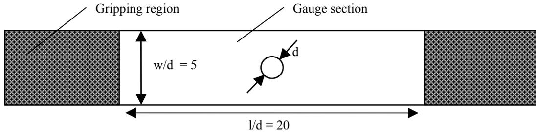
Fig. 1. Specimen Geometry
