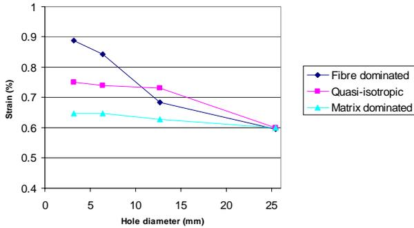
Fig. 5. Effect of layup on in-plane scaling, 0.25mm plies
