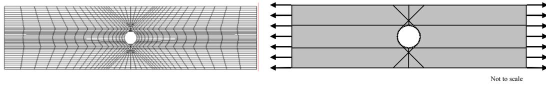
Fig. 6. Finite element mesh and location of potential split sites
