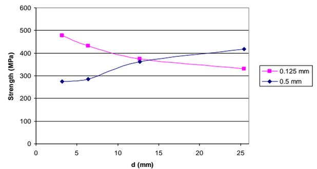
Fig. 2 Effect of ply block thickness on in-plane scaling, 4mm thick quasi-isotropic specimens
