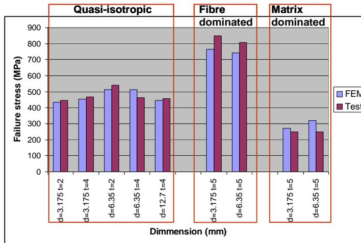
Fig. 8. Correlation of analysis and test for 0.25 mm ply specimens
