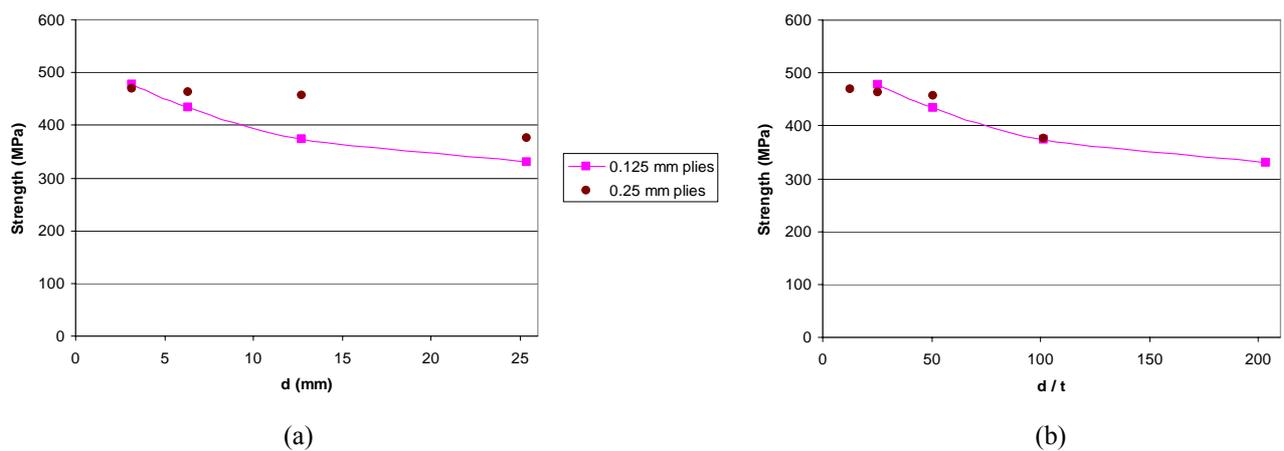
Fig. 4. Quasi-isotropic hole size effect plotted against absolute (a) and relative hole size (b)
