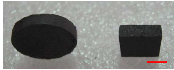
Fig.4. Samples for measuring thermal conductivity (bar: 4mm)
