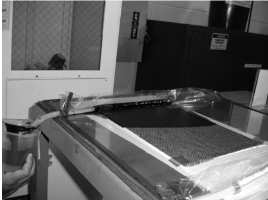
Fig. 2. Infiltration of nanotube/epoxy into a fiber preform using the VARTM process.
