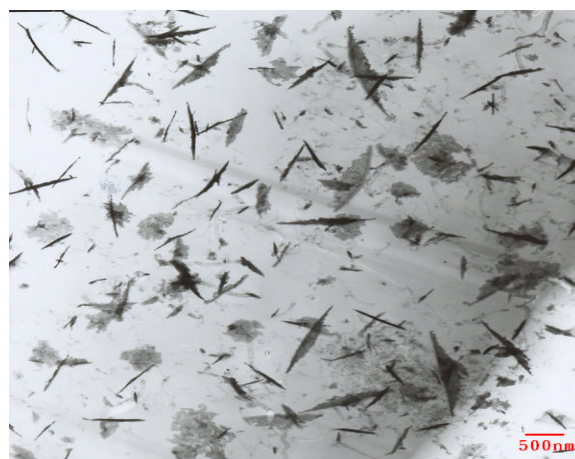
Figure 4 TEM microphotograph of VTES-MWCNT/Polyimide composites
