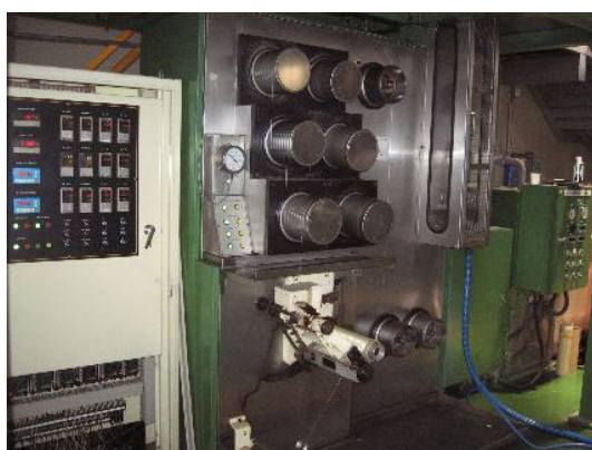
Fig. 1. Melt spinning machine used in this study.
