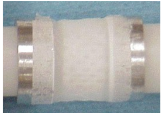
Fig. 7 Photograph of the collection of spun fiber using the rotary cylindrical electrodes at 20 min of collecting time
