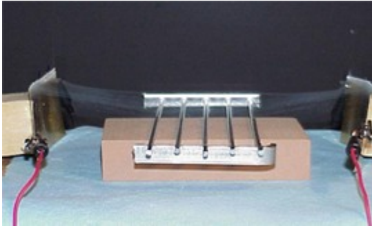
Fig.9 Deposition of aligned fibers in PLC controlled electric field
