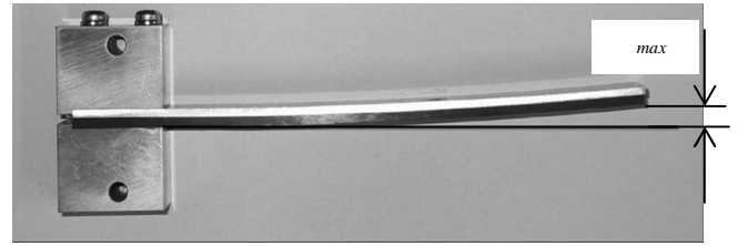
Fig.7 Deformation of the CFRP/aluminum DCB joint with 2.6mm thick aluminum plate during cool down process.
