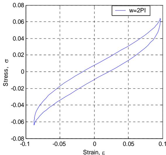
Fig. 2. Variation of stress with respect to strain for epoxy
