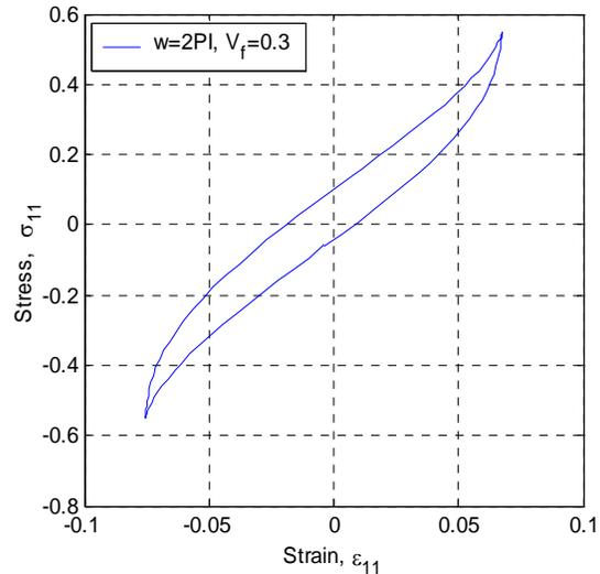
Fig. 3. Variation of stress with respect to strain for fiber volume fraction  $V_f=0.3$
