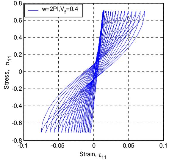
Fig 7. Variation of longitudinal stress with respect to strain for fiber volume fraction  $V_f=0.4$
