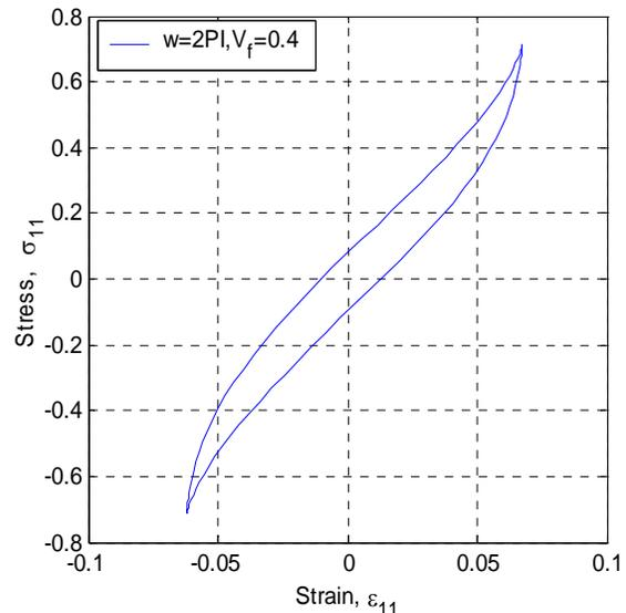
Fig. 4. Variation of longitudinal stress with respect to strain for fiber volume fraction  $V_f=0.4$
