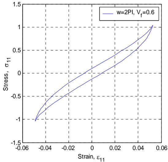
Fig 6. Variation of longitudinal stress with respect to strain for fiber volume fraction  $V_f=0.6$
