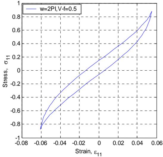
Fig. 5. Variation of longitudinal stress with respect to strain for fiber volume fraction  $V_f=0.5$
