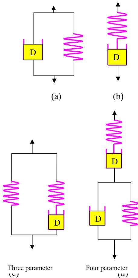
Figure 1. Two and three and four parameter model . (a) kelvin model, (b) Kelvin-Voigt model, (c) Three parameter model, (d) Four parameter model
